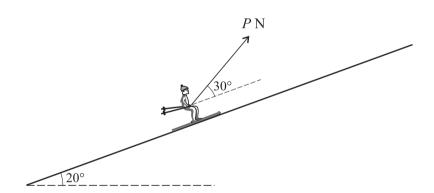
It is given that the pulling force has constant magnitude PN, and that it acts at a constant angle of  $30^{\circ}$  above the slope (see diagram). Calculate P.
