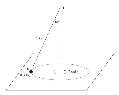
One end of a light inextensible string of length  $0.8 \,\mathrm{m}$  is attached to a fixed point A which lies above a smooth horizontal table. The other end of the string is attached to a particle P, of mass  $0.3 \,\mathrm{kg}$ , which moves in a horizontal circle on the table with constant angular speed  $2 \,\mathrm{rad} \,\mathrm{s}^{-1}$ . AP makes an angle of  $30^{\circ}$  with the vertical (see diagram).
